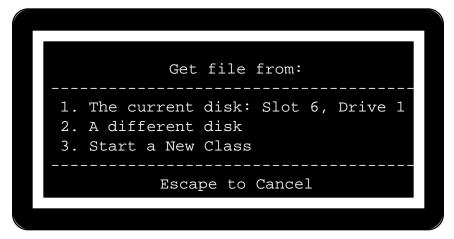
Select "3. Start a New Class" by pressing an arrow key until this option is highlighted, or press the number 3. Press <return>. You can now enter a name for the class. The program will limit you to characters that ProDOS will allow for a filename, so you don't have to worry about entering a name you shouldn't. The name can consist of up to 15 numbers, letters and periods. *It must start with a letter*. Here are some examples:
