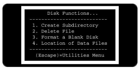
All of the disk operations with the exception of saving and opening classes are covered under this menu item. You can Create a Subdirectory, Delete a File, Format a Blank Disk, and set the Location of Data Files.
